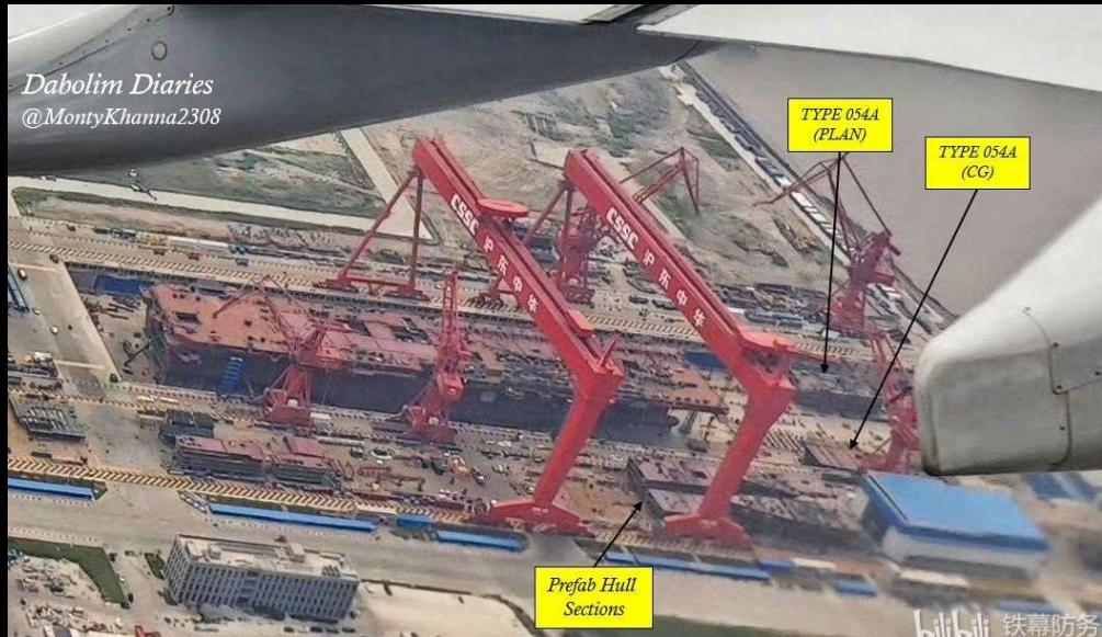
A photograph of the drydock dated 28 August 2024 taken in a flyby and posted on X by @horobeyo shows the commencement of work on the two frigates on the dock floor. The picture also shows large pre-fabricated modules of the vessels placed adjacent to the dock awaiting to be lowered and mated with the vessels. From this image, it may be assessed that formal keel laying of the vessels on the dock floor took place in mid-August 2024.
