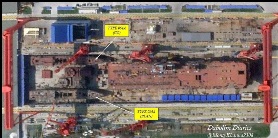
A satellite update posted on SinoDefenceForum on 08 October 2024 shows the considerable progress made in construction of the two vessels. The hulls appear to be complete with only sections of the superstructure yet to be placed on the ships.
