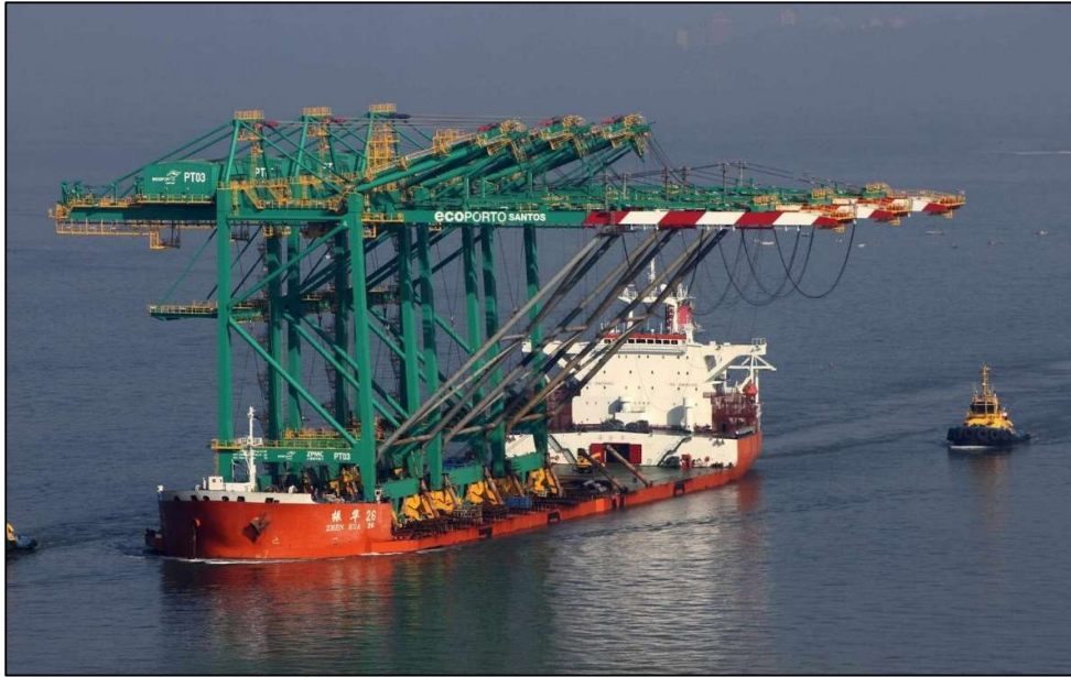
Zhen Hua 26 with Three Container Cranes Embarked
