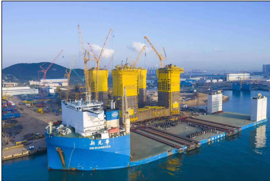
Xin Guang Hua Loading a FPSO Hull
