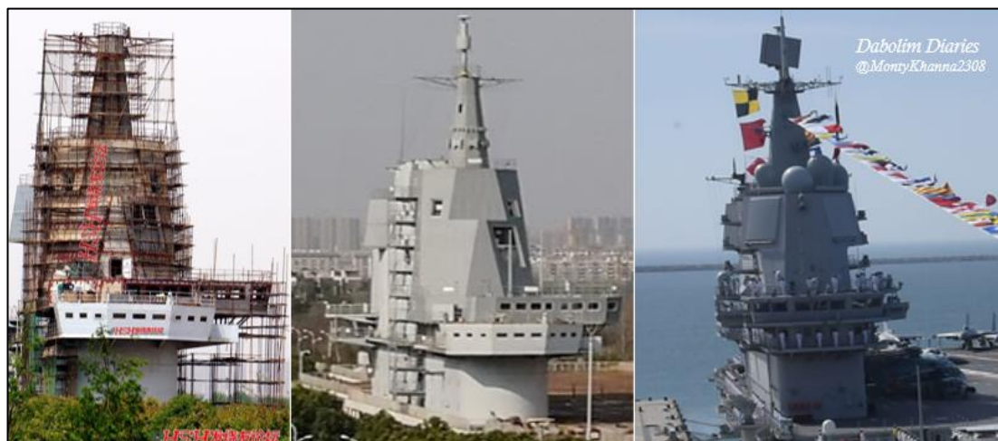
Island of Mock-Up Being Modified (Left), Completed (Center), Actual on Shandong (Right)
