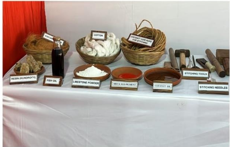
Figure 2. Traditional Materials Used for Stitched Ship Construction Source: Directorate of Naval Architecture, Indian Navy
