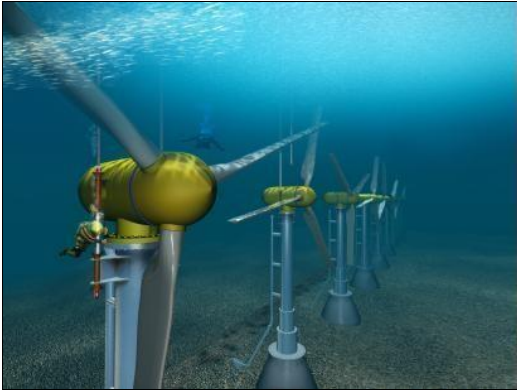
Fig 6: Underwater Horizontal-Axis Turbines Operated by Ocean Currents Source: US Department of the Interior, Bureau of Ocean Energy Management (BOEM)
