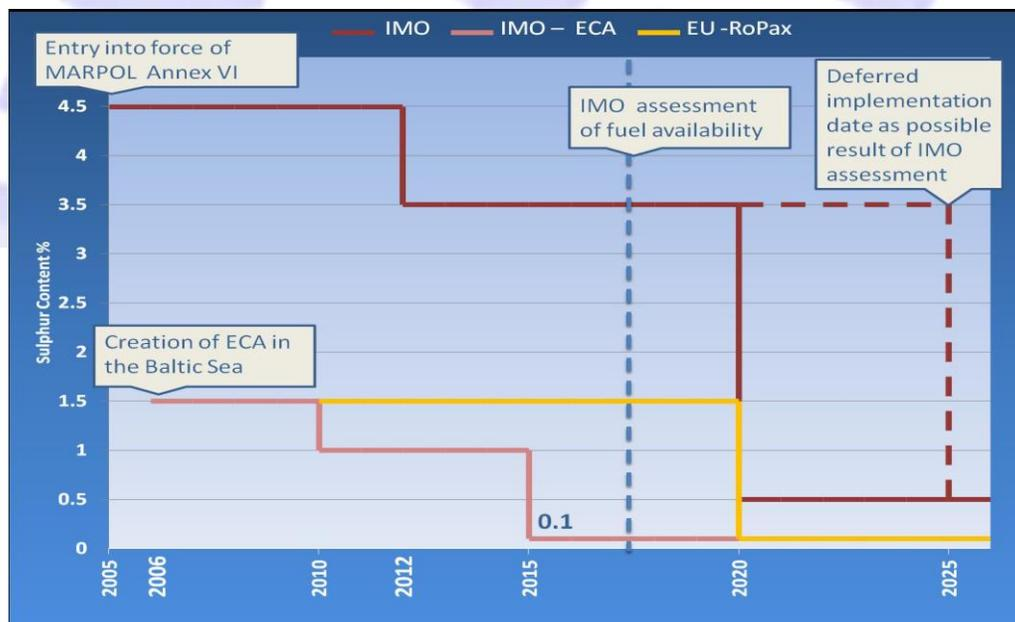
Fig 1. Allowable sulphur content in fuels used on board ships
